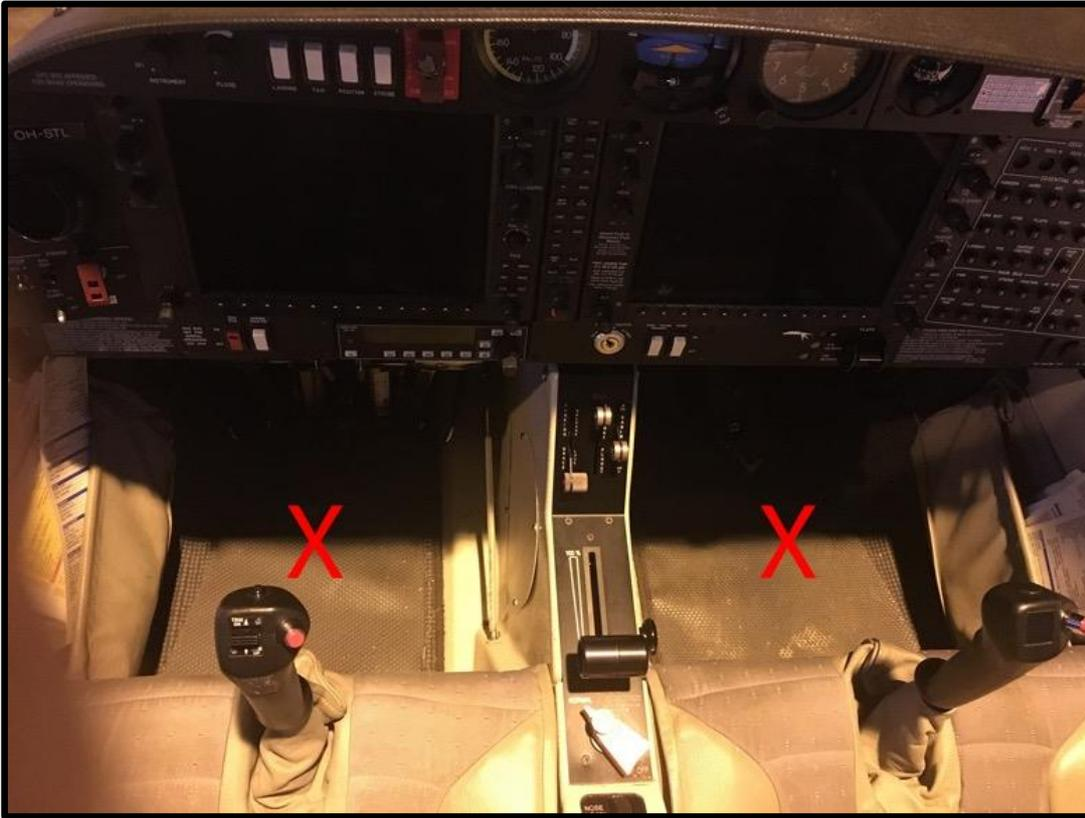
Two heaters were placed inside the cabin: one at the pilot side, one at the co-pilot side.
