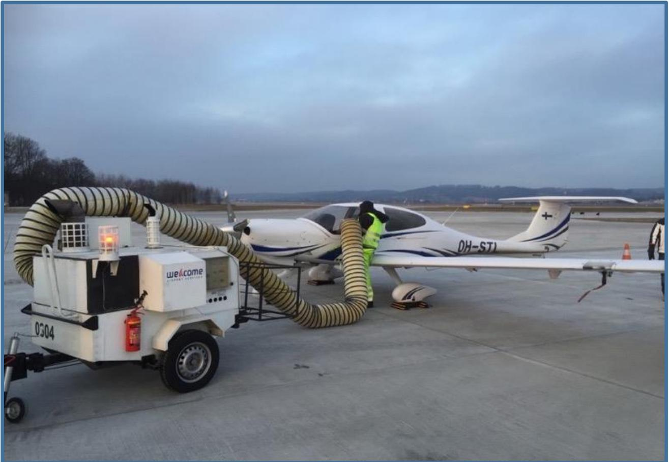
This is what happened when the plane got frozen in Krakow: the (promised) electricity was not available, and outside temperature was -15C. There were two mobile warm air generators that were used to thaw the airplane after spending the night in freezing conditions, one for the cabin and one for the engine. It took two hours to get the plane warmed up – all went well though!
