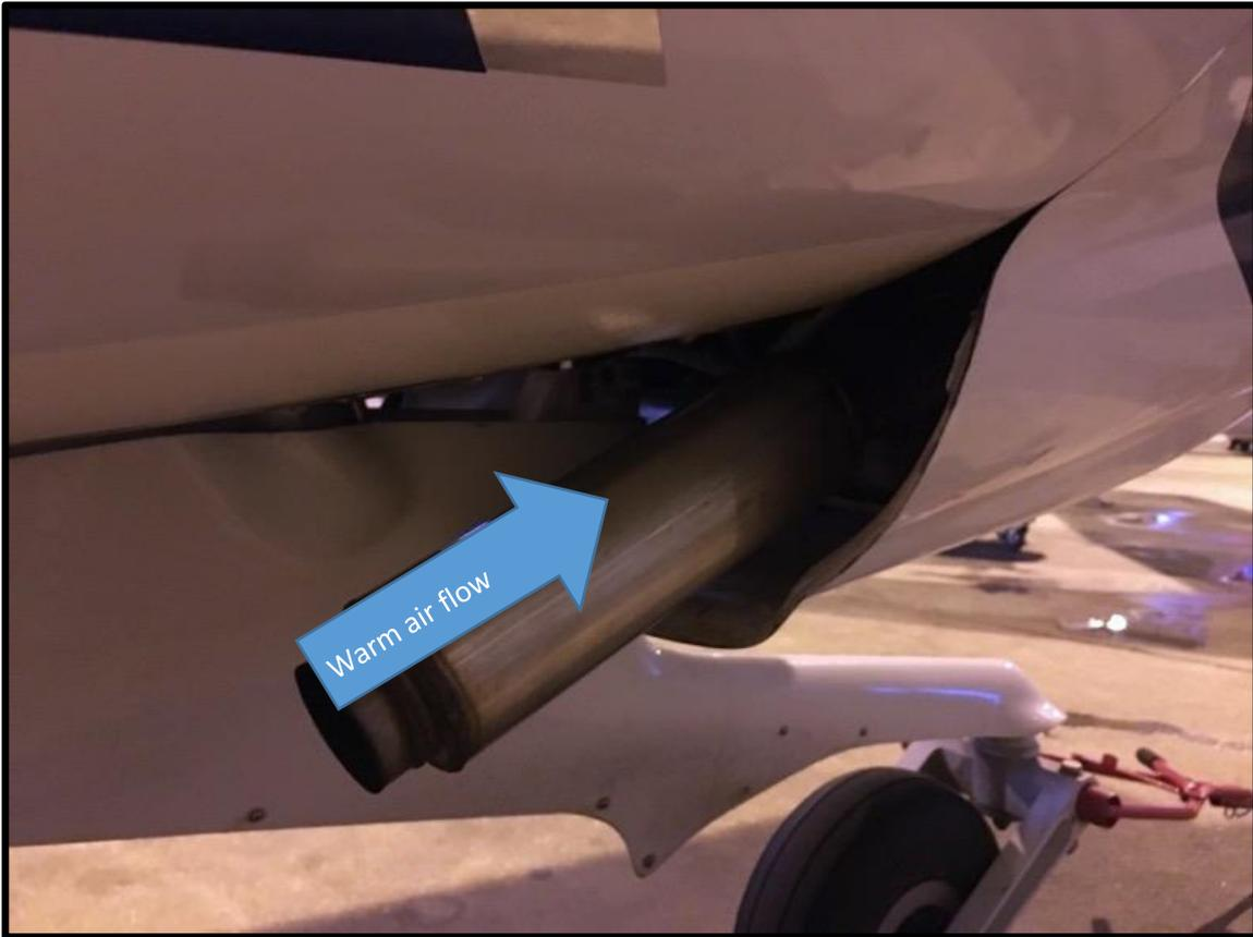
We did not use engine heater, but one could be placed underneath the plane, the air flowing toward the engine space. Add an engine cover to keep the warmth in.
