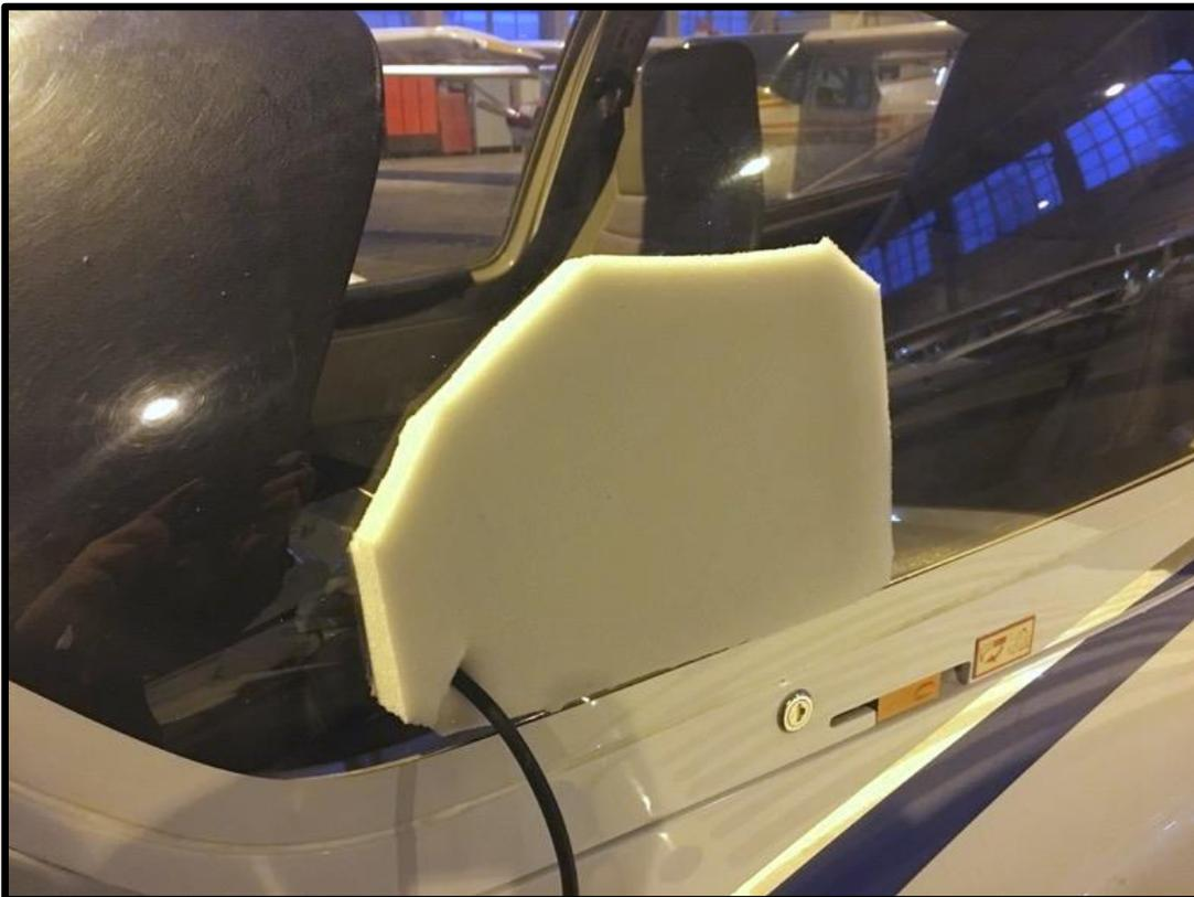
Special piece of foam "window cover" was put to the open small window, power cord pushed through the foam cut. This will keep the warmth inside and (cold) weather outside.
